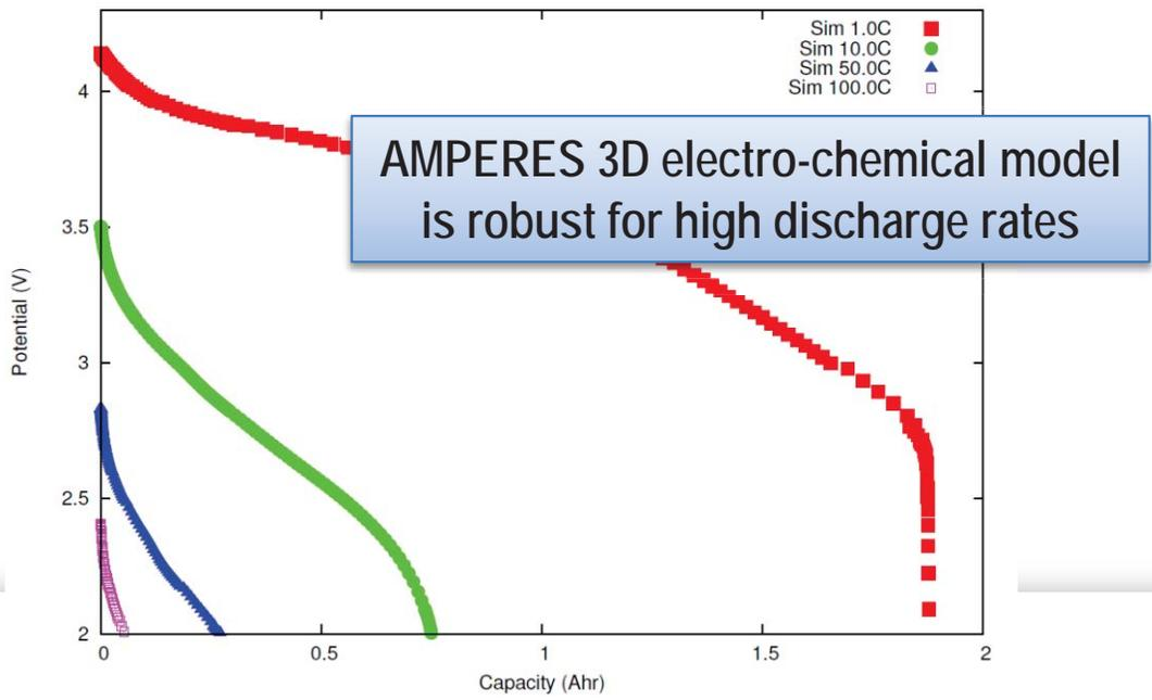
AMPERES 3D electro-chemical model is robust for high discharge rates
