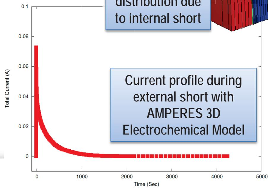
Current profile during external short with AMPERES 3D Electrochemical Model
