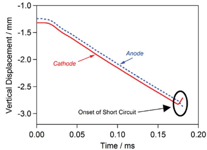
Short occurs when separator fails and cathode and anode come in contact
