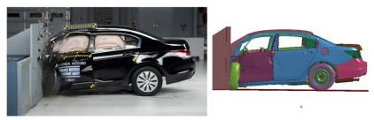
Post-test laboratory vehicle and model of the 2009 Honda Accord for IIHS SOL test
