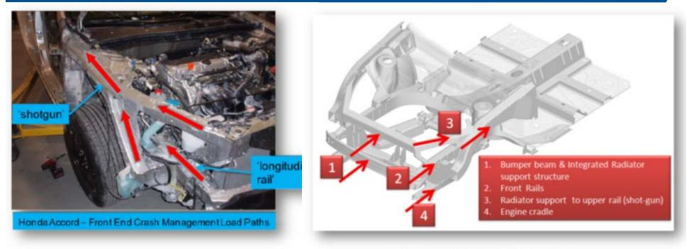
Figure 88: Honda Accord Front Structure
