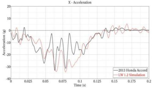
Intrusions of MY2013 Accord and the LWV 1.2 on the IIHS structural measuring scheme Crash pulse in the x-direction for the center of gravity of the MY2013 Honda Accord and the LWV 1.2 in IIHS SOL impact
