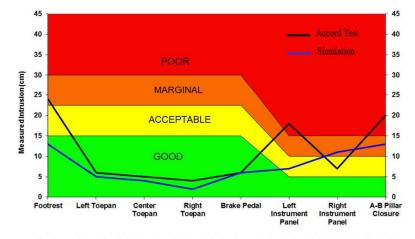
Maximum intrusion in laboratory test and finite element simulation in IIHS SOL frontal impact.
