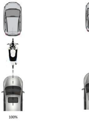
Motorcycle target positioned 2 meters behind car target
