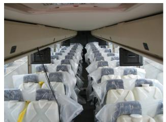
AP Figure 3. 175 lb. water Dummies were used to ballast the motorcoaches to the GPOW load condition.
