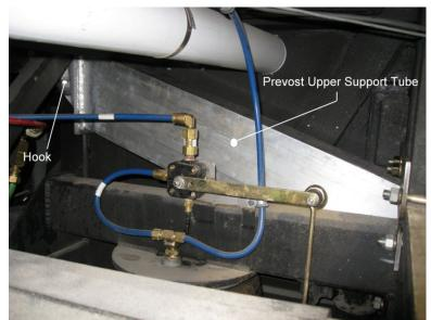
AP Figure 28. Photograph of the right side Prevost upper support tube installed.
