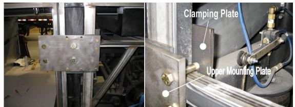
AP Figure 24. Photographs of the fabrication of the Prevost upper mounting plates. Left: Driver-side upper mounting plate bolted in place with clamping plates and the upper support Tube before the tabs were installed. Right: This photo is of the same mounting plate shows the clamping plate on the inside of the stainless steel tubing of the motorcoach and the aluminum upper support tube (center background).
